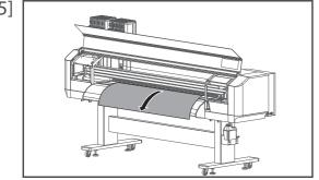
Rewind the media onto the roll to remove warp or skew. [6]
