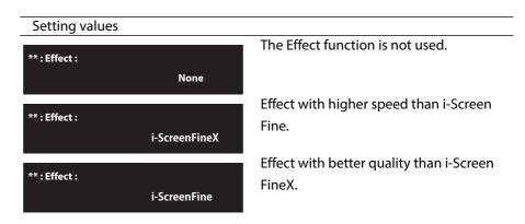
Type \*\*: 2 **Adjust Print**  Sets up when adjusting the printer for the optimum quality of image print. Before adjusting this setting, enter the thickness of the media.
