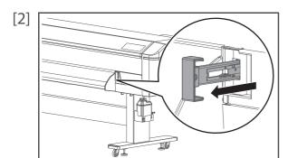
From the front side of the printer, pull the media feed lever towards you as much as possible to release the pressure rollers.
